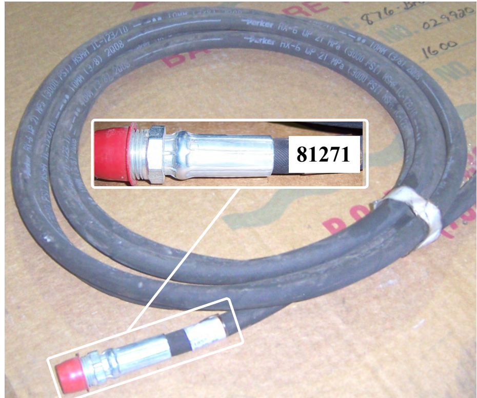
Р# 81271 Гидрошланг .25H x .25NPTMS x .56JICMS x 96" Long.
