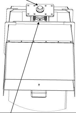
The bearing located at the end of the vertical auger should get 1 to 2 careful pumps of grease every day of constant use.
