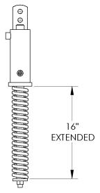
When the master is fully extended, the pressure release spring measures roughly 16" long.
