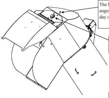
The bearing located at the end of the swivel vertical auger should get 1 to 2 careful pumps of grease every day of constant use.
