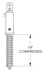
When adding braking fluid to the master cylinder for the last time, the pressure releasing spring must be held compressed at 14" long.
