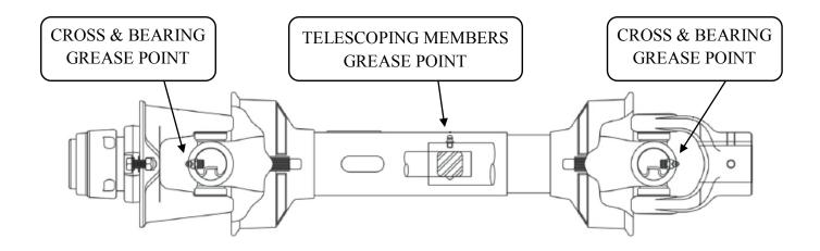
LUBRICATE ALL FITTINGS WITH A GOOD QUALITY LITHIUM SOAP BASE E.P. GREASE MEETING THE N.L.G.I. #2 SPECIFICATIONS AND CONTAINING NO MORE THAN 1% MOLYBDENUM DISULFIDE. (EX. SHELL SUPER DUTY OR EQUIVALENT)
