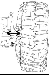
Distance measured from rim to frame rail should be adjusted to 1/16" shorter in front on both sides.
