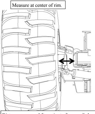
Distance measured from rim to frame rail should be adjusted to 1/16" shorter in front on both sides.
