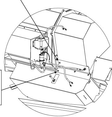
The bearing at the bottom end of the vertical auger has a grease line and fitting that permits greasing externally. This location should get 1 to 2 careful pumps of grease every day of constant use.
