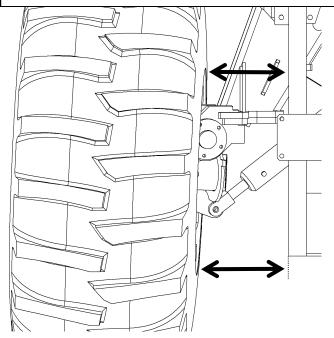
Distance measured between left and right rims should be adjusted to 1/8" shorter to the front.
