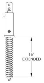
When the master is fully extended, the pressure release spring measures roughly 16" long.
