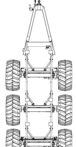
Distance measured from rim to frame rail should be adjusted to 1/16" shorter in front on both sides.
