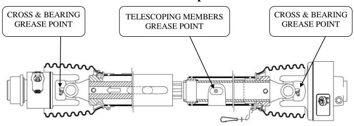
LUBRICATE ALL FITTINGS WITH A GOOD QUALITY LITHIUM SOAP BASE E.P. GREASE MEETING THE N.L.G.I. #2 SPECIFICATIONS AND CONTAINING NO MORE THAN 1% MOLYBDENUM DISULFIDE. (EX. SHELL SUPER DUTY OR EQUIVALENT)
