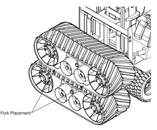
**FIGURE 5:** Use a forklift to provide support and stability when removing the straps and lifting from the top of the stack.
