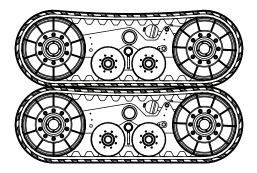
**FIGURE 2:** Tracks properly stacked on top of each other. These will freely move when the first strap is removed.
