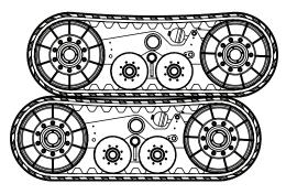
**FIGURE 3:** Tracks may shift putting additional stress on the straps making them difficult to remove.
