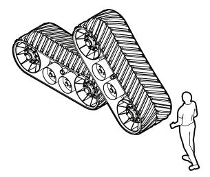
**FIGURE 4:** Unsupported tracks may roll off the stack when straps are removed.
