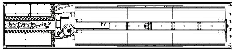
**FIGURE 1:** Tracks and extension sides are loaded to the front of the container. The main grain cart body and the extension front and back panels are loaded in the back of the container.
