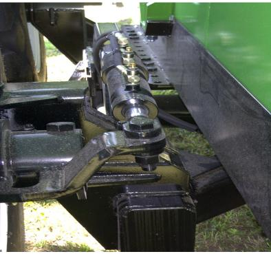
Do not open petcocks unless bleeding the system. Opening petcocks can allow air to enter the system, which will cause improper steering action.
