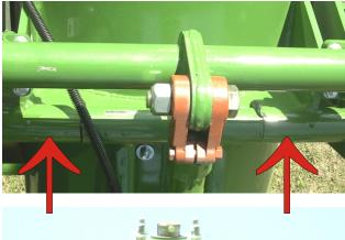
Two grease fittings are located on the auger folding hinge. These should be greased every day. Pump grease until old grease is visible.
