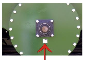
The bearing at the rear end of the horizontal auger. This location should get 1 to 2 careful pumps of grease every 2 day of constant use. Excessive pressure applying grease can be harmful to the bearing seals.
