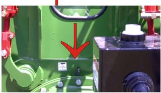
The middle bearing for the horizontal auger has a grease line and fitting that permits greasing externally. This location should get liberal greasing every 3 hours of constant use in normal conditions. In dusty or dry conditions more frequent greasing is recommended.
