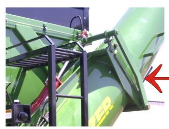
The mid bearing on the vertical auger has a grease fitting that is accessible with the auger folded. Grease at this location liberally every day of operation under normal conditions and more frequent if dusty or hot.
