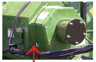
The bearing at the front end of the horizontal auger has a grease line and fitting that permits greasing externally. This location should get 1 to 2 careful pumps of grease every day of constant use. Excessive pressure applying grease can be harmful to the bearing seals.
