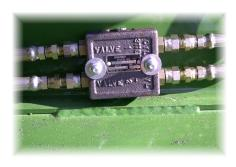
This valve prevents the auger from falling if the hose to the tractor would accidentally get ruptured. It also acts as a lock once auger is unfolded, preventing possible oil, seepage back to the tractor. It also has flow restrictions which control the speed that the auger unfolds. If the speed is inadequate, consult Balzer for recommendations.
