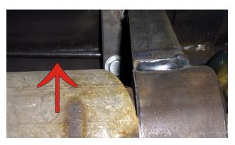
Middle horizontal auger bearing, arrow is pointing to grease line which runs to front of grain cart.
