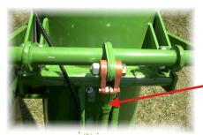
This provides a mean of adjustment if needed. Hydraulic cylinder must be completely extended and hinge totally closed. See trouble shooting for more informations.
