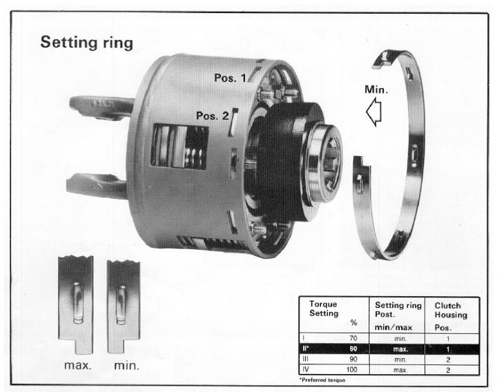
The torque setting can be modified with the aid of a setting ring and two alternative location slots in the clutch housing.
