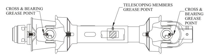
LUBRICATE ALL FITTINGS WITH A GOOD QUALITY LITHIUM SOAP BASE E.P. GREASE MEETING THE N.L.G.I. #2 SPECIFICATIONS AND CONTAINING NO MORE THAN 1% MOLYBDENUM DISULFIDE. (EX. SHELL SUPER DUTY OR EQUIVALENT)
