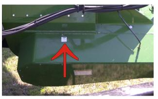
The bearing at the bottom end of the vertical auger has a grease line and fitting that permits greasing externally. This location should get 1 to 2 careful pumps of grease every day of constant use. Excessive pressure applying grease can be harmful to the bearing seals.
