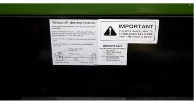
Proper steering is dependant upon adequate greasing. When conditions are dry and dusty, the tandem arms and kingpins will require grease more often.
