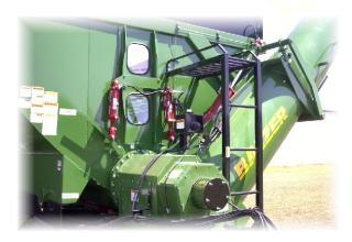
The hydraulic hoses with orange marking band control the vertical auger folding.
