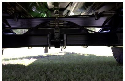
Grease fittings are located in two positions on tandem arms at the bottom of the round center pivot tube.
