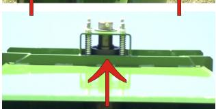
The bearing located at the end of the vertical auger should get 1 to 2 careful pumps of grease every day of constant use. Excessive pressure applying grease can be harmful to the bearing seals.
