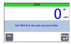
2. Follow the prompt and place test weight (the weight you entered) on the scale and press the **Enter** key.
