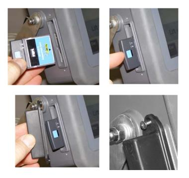
Figure 10.1 Installing the Compact Flash radio
