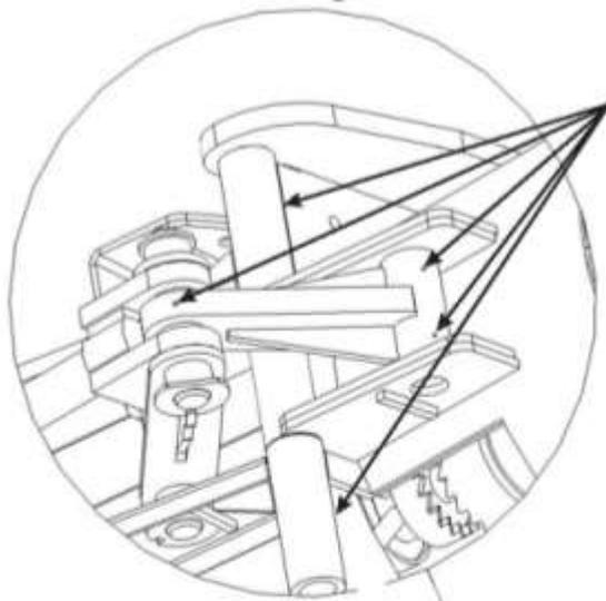
Five (5) grease fittings are located on the auger folding hinge. These should be greased every day. Pump grease until old grease is visible.
