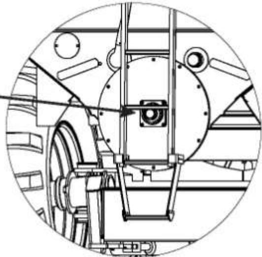
The middle bearing for the horizontal auger has a grease line and fitting that permits greasing externally. This location should get a liberal greasing after every 4 hours of constant use in normal conditions. In dusty or dry conditions, more frequent greasing is recommended.
