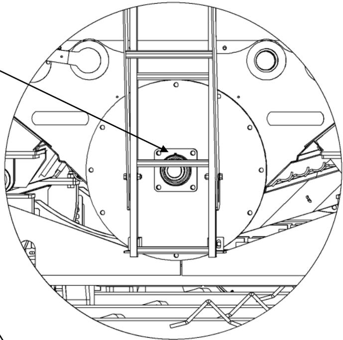
The bearing at the front end of the horizontal auger has a grease line and fitting that permits greasing externally. This location should get 1 to 2 careful pumps of grease every day of constant use.
