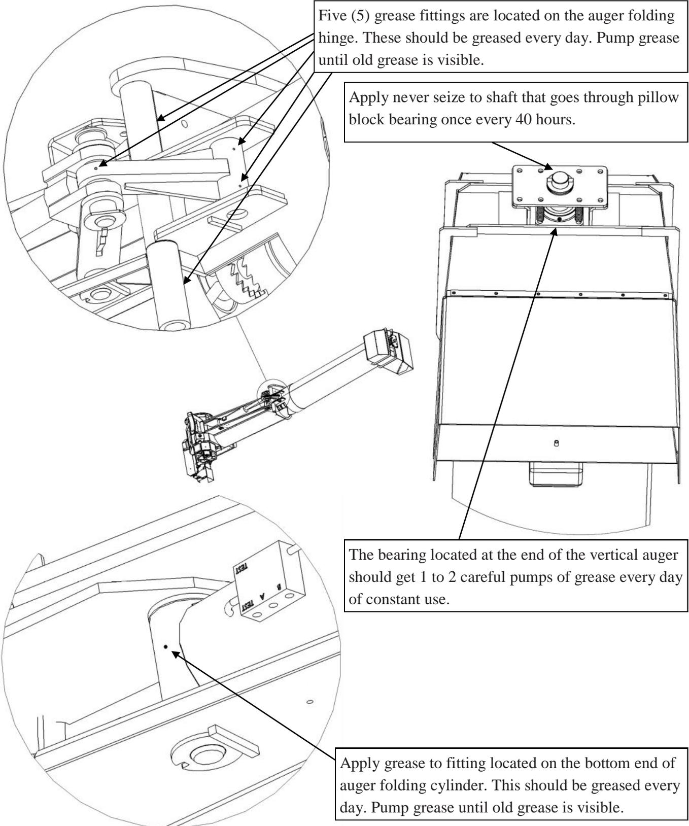
Five (5) grease fittings are located on the auger folding hinge. These should be greased every day. Pump grease until old grease is visible.
