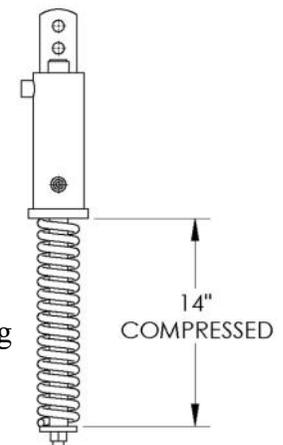
When adding braking fluid to the master cylinder for the last time, the pressure releasing spring must be held compressed at 14” long.
