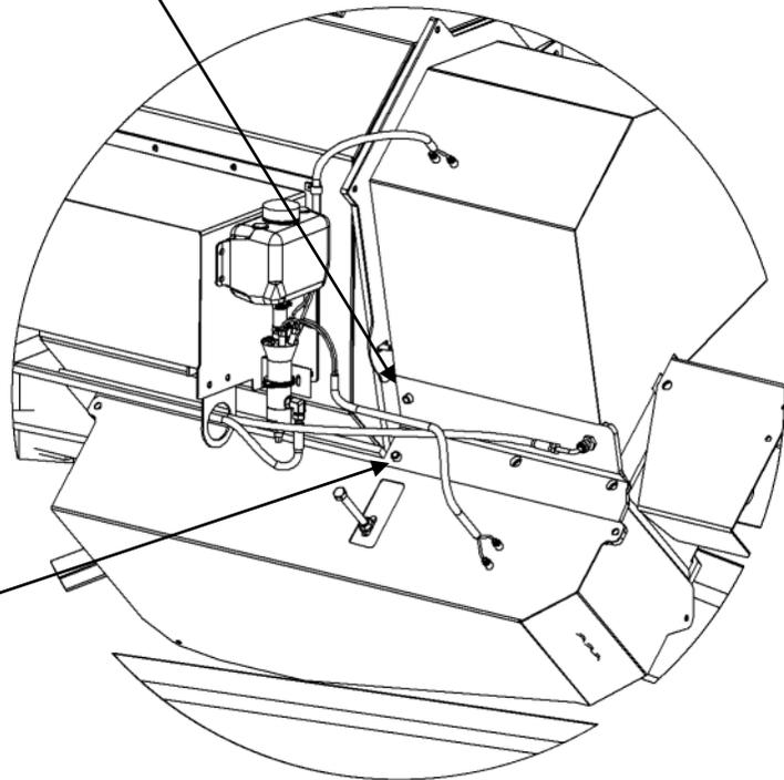
The bearing at the bottom end of the vertical auger has a grease line and fitting that permits greasing externally. This location should get 1 to 2 careful pumps of grease every day of constant use.
