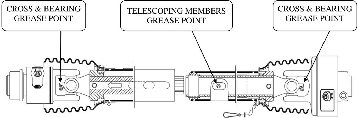
LUBRICATE ALL FITTINGS WITH A GOOD QUALITY LITHIUM SOAP BASE E.P. GREASE MEETING THE N.L.G.I. #2 SPECIFICATIONS AND CONTAINING NO MORE THAN 1% MOLYBDENUM DISULFIDE. (EX. SHELL SUPER DUTY OR EQUIVALENT)
