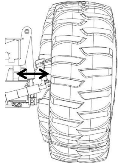
Distance measured from rim to frame rail should be adjusted to  $1/16''$  shorter in front on both sides.
