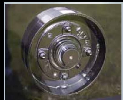
Double row spherical rotor bearing
