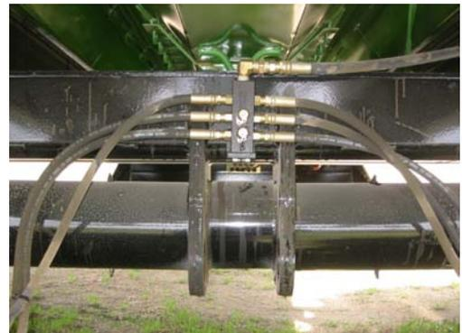
Grease fittings are located at the top and bottom of the steering hinge kingpins.
