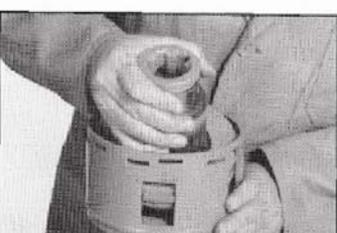
2. Insert the flange hub with friction disks and drive plates into the clutch housing - lining up the tabs of the drive plate.
