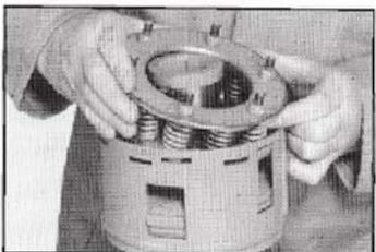
4. Lift the spring pack assembly out by tilting it up opposite the locating tab which is on the bottom plate of the spring pack.
