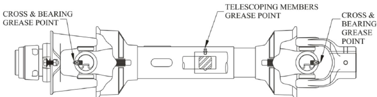
LUBRICATE ALL FITTINGS WITH A GOOD QUALITY LITHIUM SOAP BASE E.P. GREASE MEETING THE N.L.G.I. #2 SPECIFICATIONS AND CONTAINING NO MORE THAN 1% MOLYBDENUM DISULFIDE. (EX. SHELL SUPER DUTY OR EQUIVALENT)
