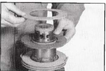
1. Fit friction disks and drive plates to flange hub in correct sequence as illustrated. One friction disk is mounted in the bottom of the clutch housing along with the fiber hub pilot bearing.
