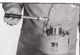
5. Back off the 6 nuts to the end of the studs. In this position the spring pack is at the pressure controlled by the location of the setting ring.
