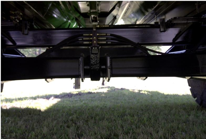
Grease fittings are located in two positions on tandem arms at the bottom of the round center pivot tube.
