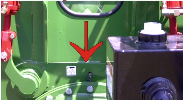
The middle bearing for the horizontal auger has a grease line and fitting that permits greasing externally. This location should get liberal greasing every 3 hours of constant use in normal conditions. In dusty or dry conditions more frequent greasing is recommended.
