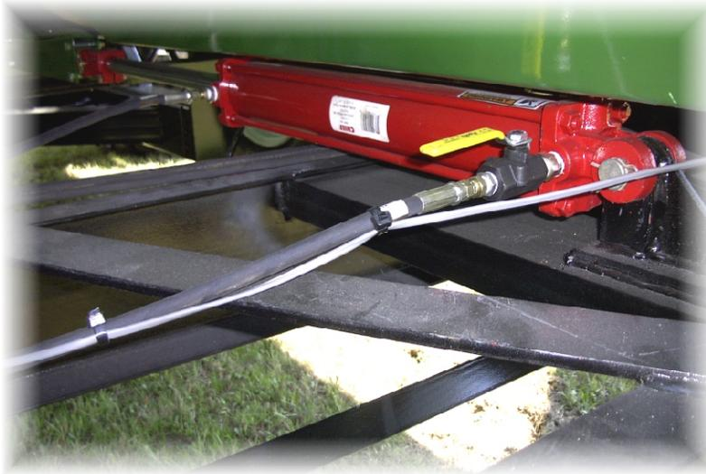
The picture below shows the hydraulic cylinder which control the clean-out doors. A valve is provided which when closed prevents these doors from accidental opening.
