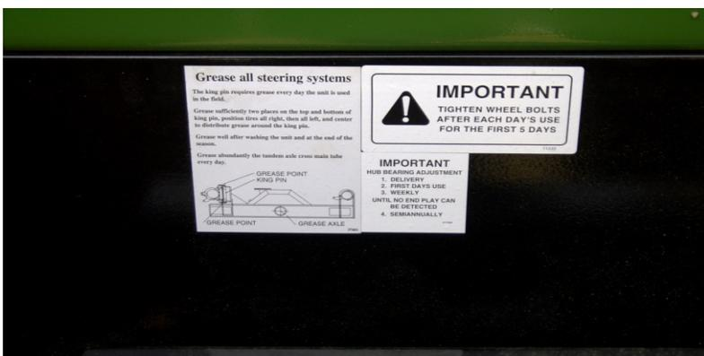
Proper steering is dependant upon adequate greasing. When conditions are dry and dusty, the tandem arms and kingpins will require grease more often.
