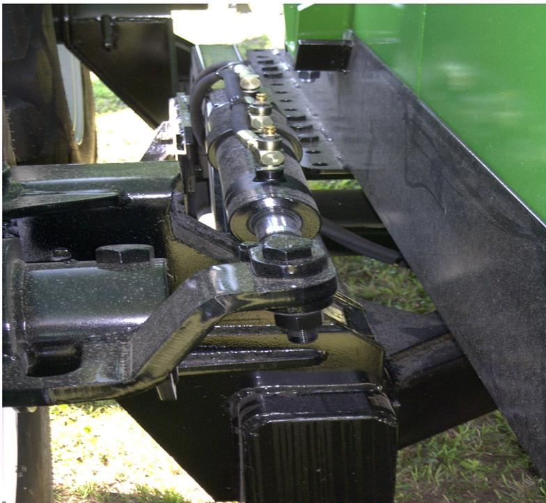
Do not open petcocks unless bleeding the system. Opening petcocks can allow air to enter the system, which will cause improper steering action.
