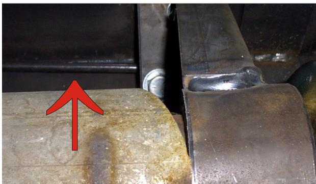
Middle horizontal auger bearing, arrow is pointing to grease line which runs to front of grain cart.
