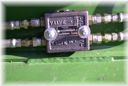
This valve prevents the auger from falling if the hose to the tractor would accidentally get ruptured. It also acts as a lock once auger is unfolded, preventing possible oil, seepage back to the tractor. It also has flow restrictions which control the speed that the auger unfolds. If the speed is inadequate, consult Balzer for recommendations.
