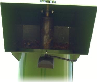
The upper bearing is spring loaded to allow auger to ride up as the lower and upper augers engage. It must return to its proper position as power is applied.
