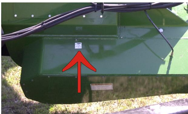
The bearing at the bottom end of the vertical auger has a grease line and fitting that permits greasing externally. This location should get 1 to 2 careful pumps of grease every day of constant use. Excessive pressure applying grease can be harmful to the bearing seals.
