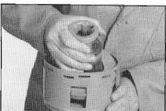
2. Insert the flange hub with friction disks and drive plates into the clutch housing - lining up the tabs of the drive plate.
