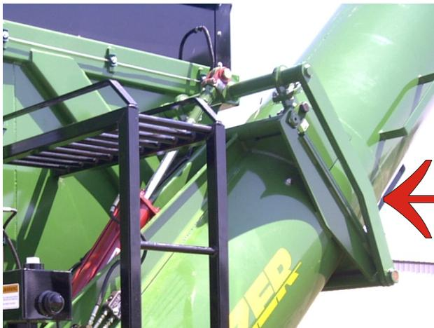
The mid bearing on the vertical auger has a grease fitting that is accessible with the auger folded. Grease at this location liberally every day of operation under normal conditions and more frequent if dusty or hot.
