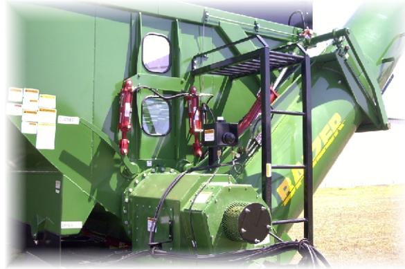
The hydraulic hoses with orange marking band control the vertical auger folding.
