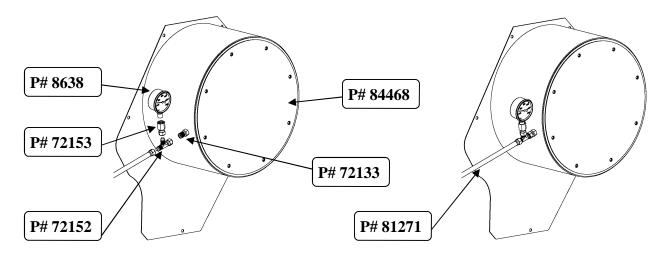
Connect T-fitting **P# 72152** to bulkhead fitting **P# 72133**. Connect JIC Female adapter **P# 72153**. Connect pressure gauge **P# 8638** to female adapter using Teflon thread tape. Re-connect hydraulic hose **P# 81271**. Tighten all connections.
