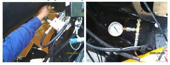
Inform the operator to engage the tractor valve to the Float position (Note: This does not mean the Neutral Position on the tractor valve.) "Clutch should be Disengaged" when auger is not unloading, and more importantly before shutting down the tractor. Trapped oil in the clutch circuit can expand due to warm air temperatures, causing the swivel fitting to fail.
