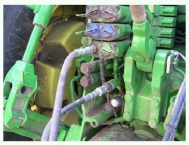
THE UPPER LINE CONNECTS TO ONE OF THE TRACTOR VALVE BANK SECTION (OIL TO THE CART)
