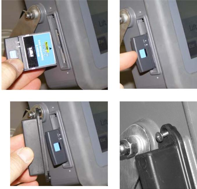
**Figure 10.1 Installing the Compact Flash radio**
