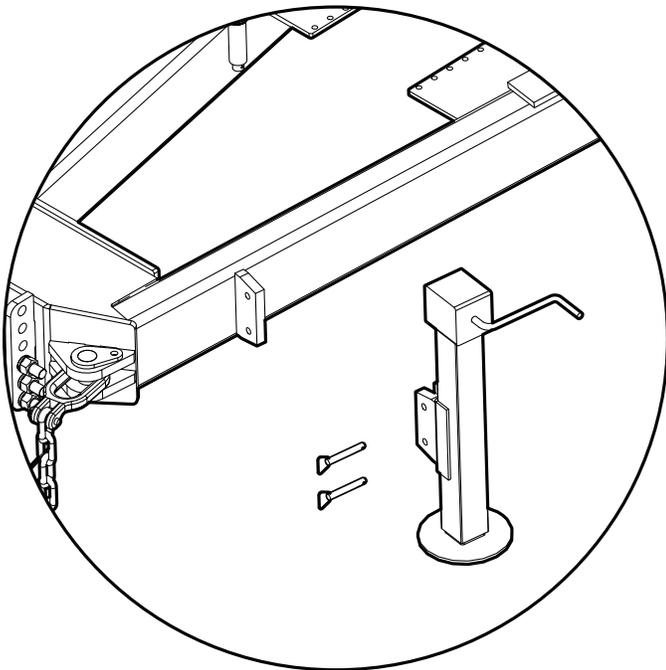
Remove pins and pull the jack off of the support tab.
