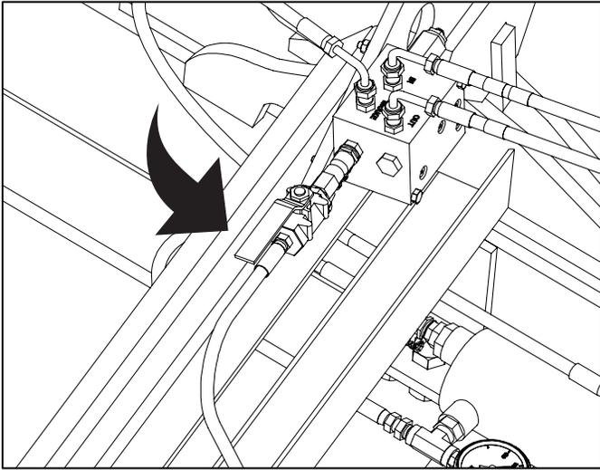
To open the ball valve on the Bleeder Hose, rotate the handle so that it is inline with the hose.
