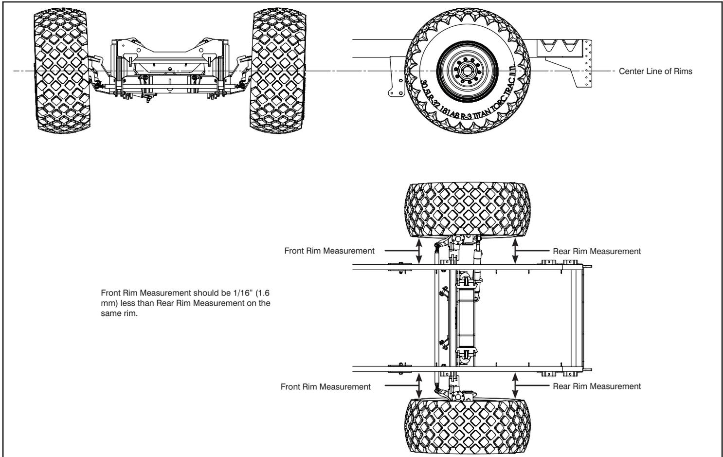
8. The inside front measurement should be 1/16" (1.6 mm) shorter than the inside rear measurement.
