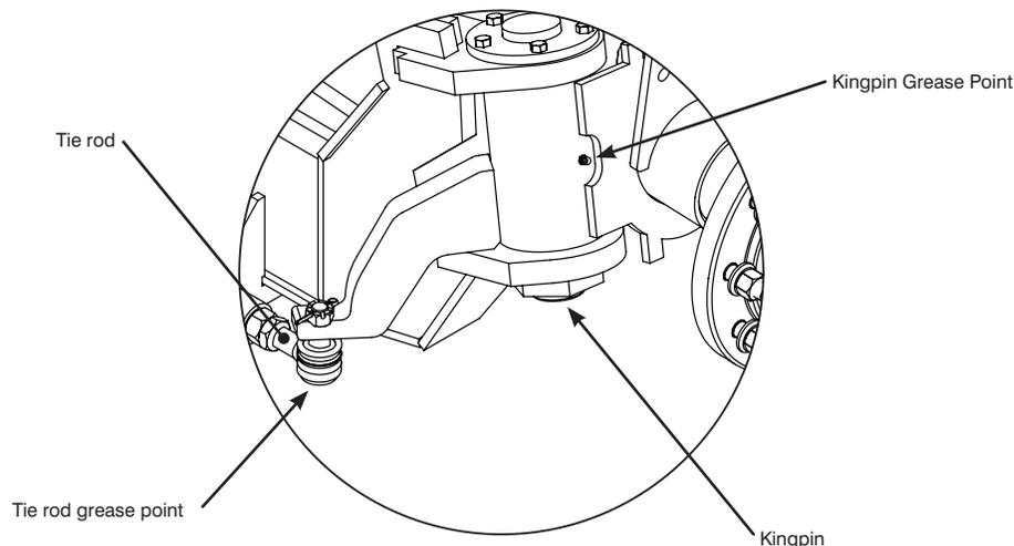
Apply grease to both grease points on the tie rod and the kingpin grease point on each wheel. If the kingpin grease point is connected to a grease line, the grease point is located on the right side rear of the frame. If there is no kingpin grease point, the kingpin has a poly bushing and does not need any grease.
