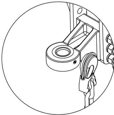
Grease points on both sides of Bull Pull hitch.
