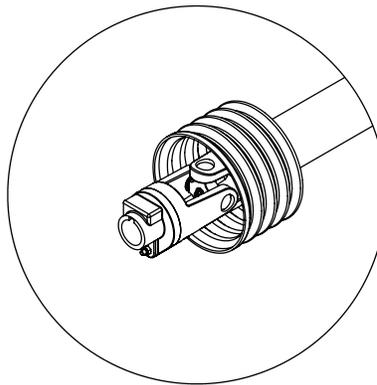
Grease points on both universal joints of the PTO shaft and on the shaft itself.
