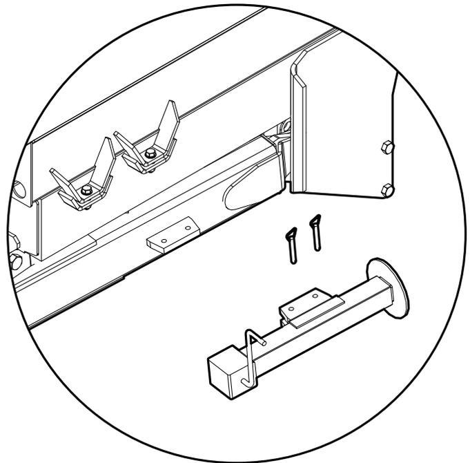
Slide jack onto storage tab and re-insert pins.
